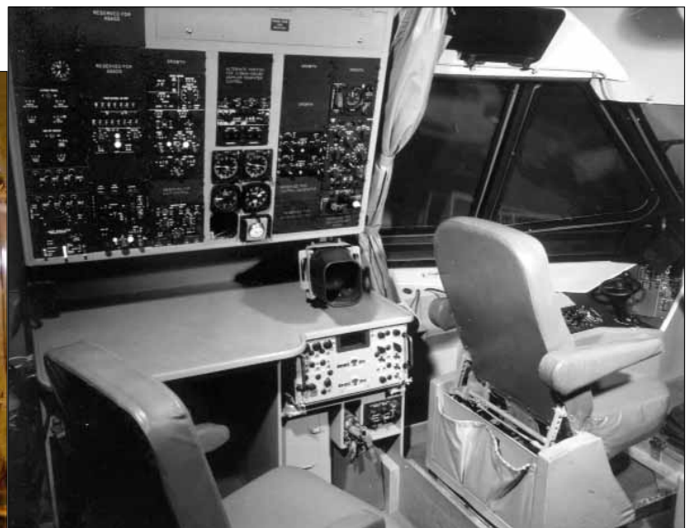
Navigator's console located behind the pilot. Also note the nose-steering control wheel on the console to the left of the pilot's seat. (Photo from Lockheed Martin)
