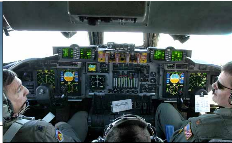
The C-141C model modifications included the installation of a glass-cockpit, seen here with a 445th MAW crew at the controls. (Lockheed Martin photo)
