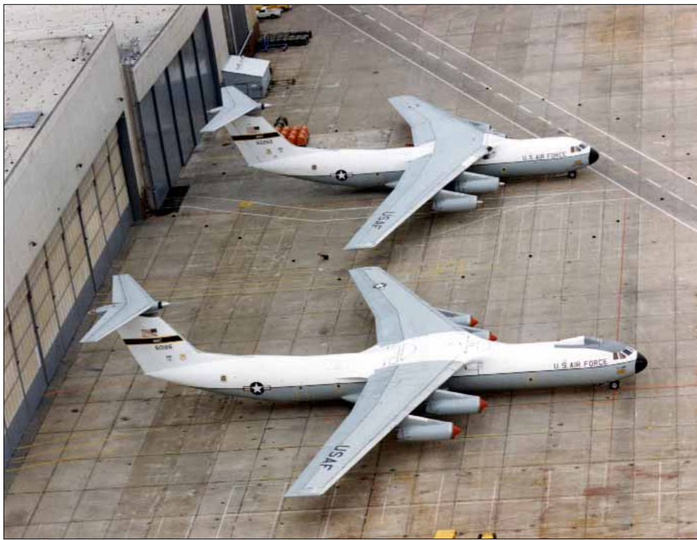
The noticeable differences between the original "A" model and converted "B" are evident in this photo clearly showing the fuselage stretch and refueling receptacle above and behind the cockpit. Ship 66-0186 is in the foreground with 65-0269 in the back. (Lockheed Aircraft photo)
