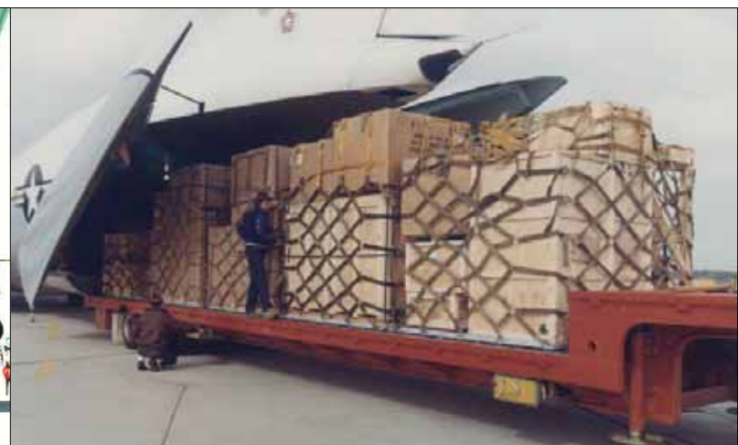
Palletized cargo loading was accommodated by the use of specially designed transport trailers facilitating "roll-on, roll-off" capabilities. (Photo provided by Lockheed Martin)
