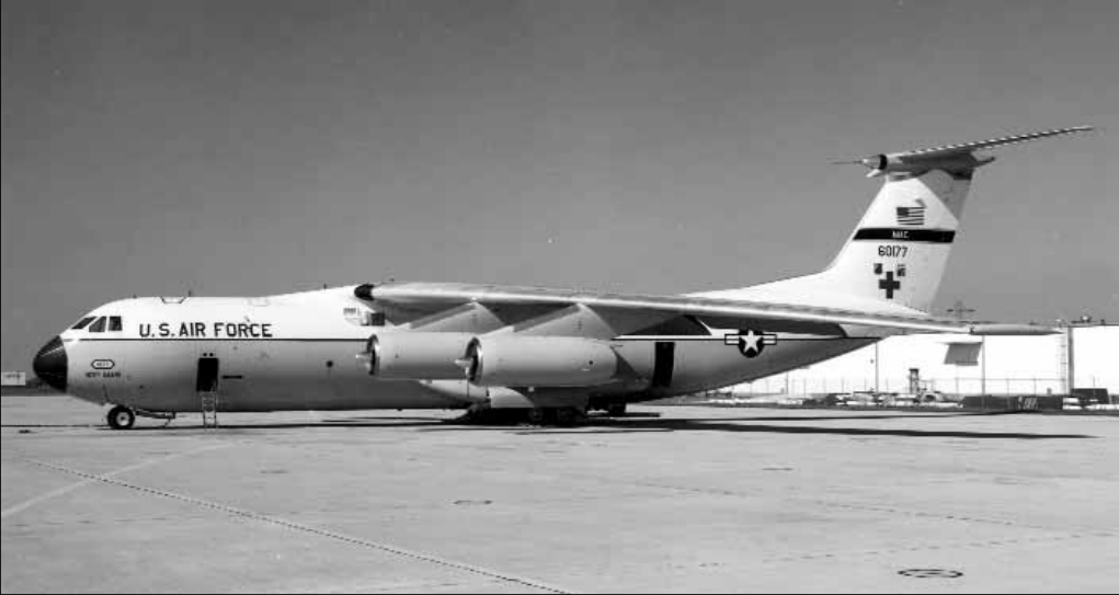
A photo of 66-0177, in "A" model form being operated by the 63rd MAW, taken shortly after its historic Hanoi flight. The aircraft is still displaying the Red Cross on the tail used for all the repatriation flights. The C-141 went through a series of paint schemes; from bare metal, to the white and gray shown here, a camouflage pattern known as European One and eventually a "Proud Gray." (USAF photo from the Paul Minert collection)
