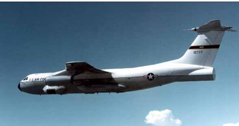
The third pre-production aircraft, 61-2777, was assigned to the 1111th TS. The aircraft was nicknamed "The Gambler." It served as a test bed for a number of electronic systems including side-scan radar (seen on the fuselage under the engine) and ECM systems for the B-1 and B-2 that were mounted in the specially modified cylindrical aft fuselage extension. (USAF photo from the Paul Minert collection)
