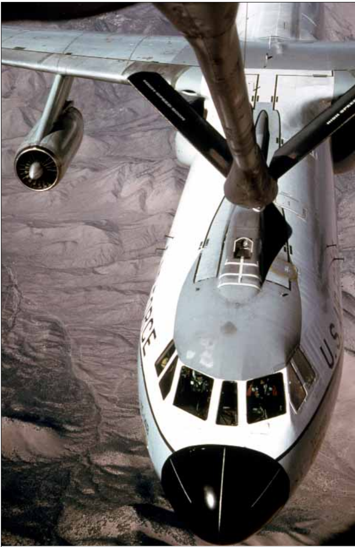
Inflight refueling capabilities added to the C-141Bs extended the aircraft's range capabilities to a truly global reach. Here YC-141B, 66-0186, is seen from the refueler's window on a KC-135 during flight testing of this aspect. (Lockheed Aircraft photo)
