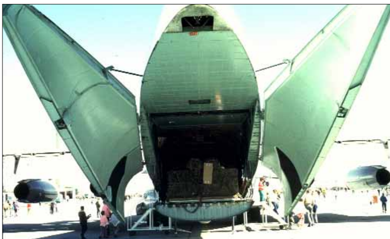
The huge "clamshell" doors to the cargo hold provided the USAF with the capability to transport both palletized cargo and bulky equipment. (From the AAHS Photo Library)
