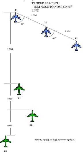
**NOTE:** Rendezvous is accomplished in the same manner regardless of the number of tankers or receivers. Figures are only used to demonstrate the positions of tankers or receivers if they are present.
