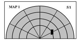
**NOTE:** This diagram depicts the position of the lead tanker when receiver one (R1) is in the proper post air refueling position (2-NM 60 degree echelon).
