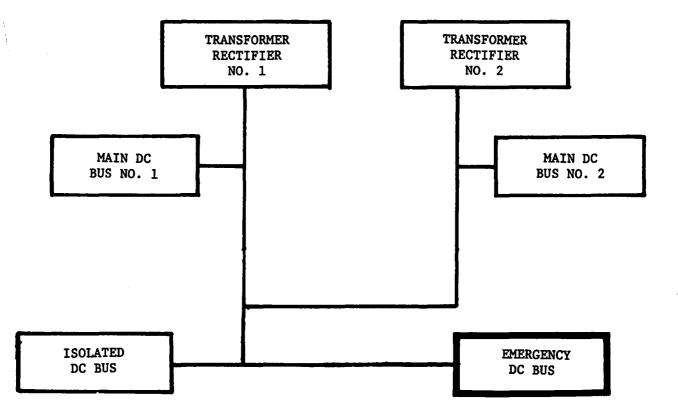
There are three more DC Buses. Remember the Avionics Circuit Breaker Panel above the Navigator's Station? On this panel, we will find two (2) MAIN DC AVIONICS BUSES and one (1) ISOLATED DC AVIONICS BUS.
