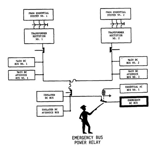
You notice that we added a *relay* in the wiring to the Emergency DC Bus. This relay is called the Emergency Bus Power Relay and *selects* either *normal* or *emergency* power for the Emergency DC Bus. This relay is normally energized closed by Essential AC Bus No. 1 as shown.
