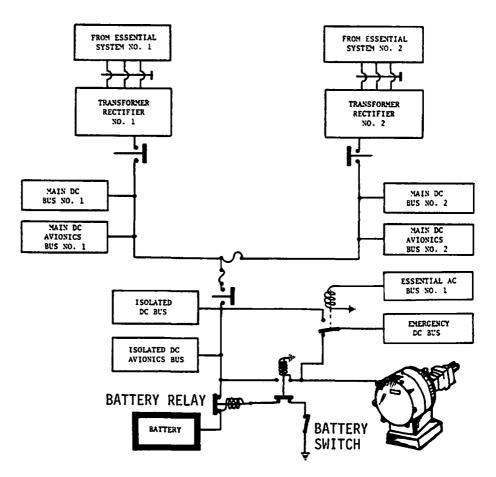
In the above diagram, NO engines are running, NO External or Auxiliary power is connected and the Battery Switch is "ON." Will the Emergency DC Bus receive power?
