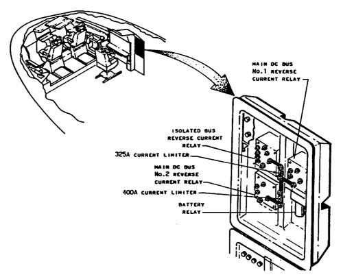
Look at the picture above and list the six DC components located behind the Flight Engineer's Circuit Breaker Panel No. 3.
