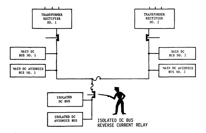
Why do you think the Isolated DC Bus Reverse Current Relay was placed between the Main DC Buses and Isolated Buses?
