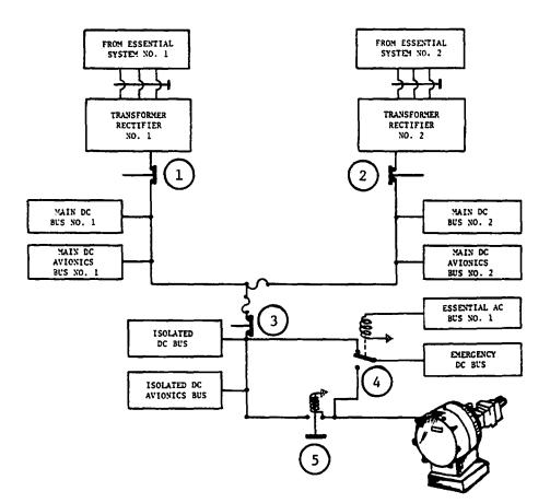
Now--the latest with the leastest - a 24 volt, 11 ampere-hour lead-acid BATTERY *located* by the Under Deck Electrical Equipment Rack forward of the crew latrine. The Battery Switch on the electrical control panel *controls* the Battery Relay which connects the BATTERY to the Isolated DC Bus and the Isolated DC Avionics Bus. Battery power is used primarily for APU starting control. The diagram below shows how the BATTERY connects to the system.
