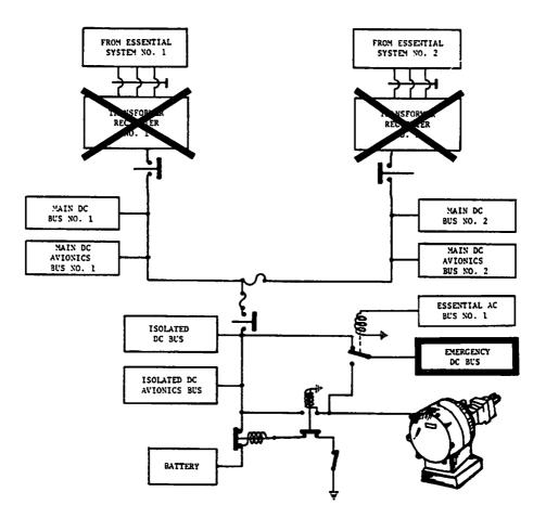
Now that we know the BATTERY will power the Emergency DC Bus if you lose both Transformer/Rectifiers and normal AC power is still available, let's locate the BATTERY and Transformer/Rectifiers. To effectively troubleshoot the system, we should know where the units are physically located. The BATTERY and TRANSFORMER/RECTIFIERS are on/or by the UNDERDECK ELECTRICAL EQUIPMENT RACK.
