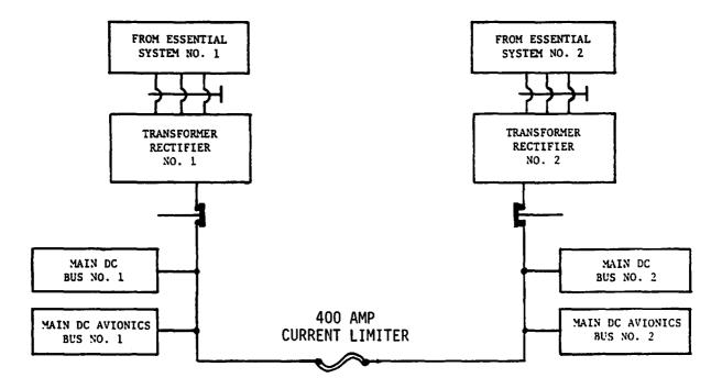
Now you can see if *either* Transformer/Rectifier *fails*, the *other can feed* the Main DC Bus through the 400 Amp Curren Limiter.
