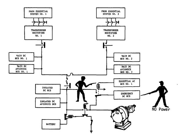
Now can we say that the BATTERY will power the Isolated DC Buses for APU starting when no other power is on the aircraft?
