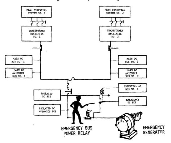
Does it seem logical that the Emergency Generator would also be the emergency power source for the Isolated DC Bus and Isolated DC Avionics Bus? ( ) Yes.
