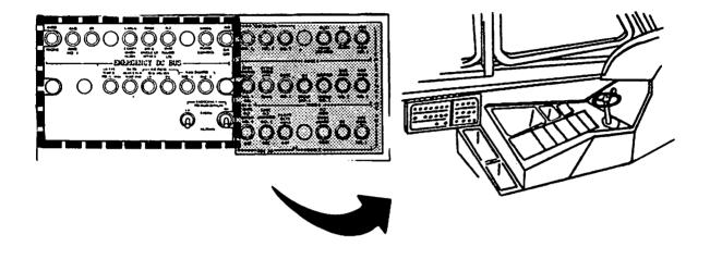
The EMERGENCY DC BUS is located on the Emergency Circuit Breaker Panel, to the left of the pilot.
