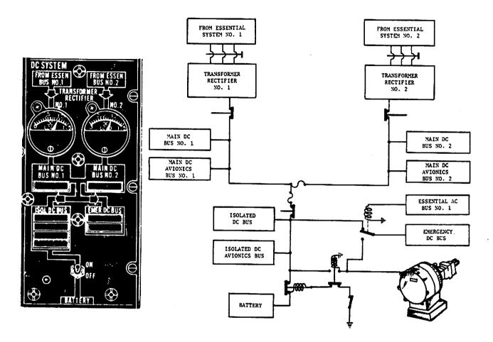
The first big *difference* that you will notice is probably the addition of *loadmeters* so that we can tell the load on each Transformer/Rectifier Unit. If you remember the rating of our Transformer/Rectifiers you should have no difficulty with this question.
