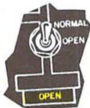
When the "Bus Tie Open" light illuminates the Flight Engineer should check the *voltage* and *frequency* of that generator. If the voltage and frequency are within limits the Bus Tie should be reset. If the "Bus Tie Open" light illuminates again NO further attempt should be made to reset. If the voltage and frequency are NOT within limits, the Generator Control Switch should be turned OFF and the BUS TIE RESET.
