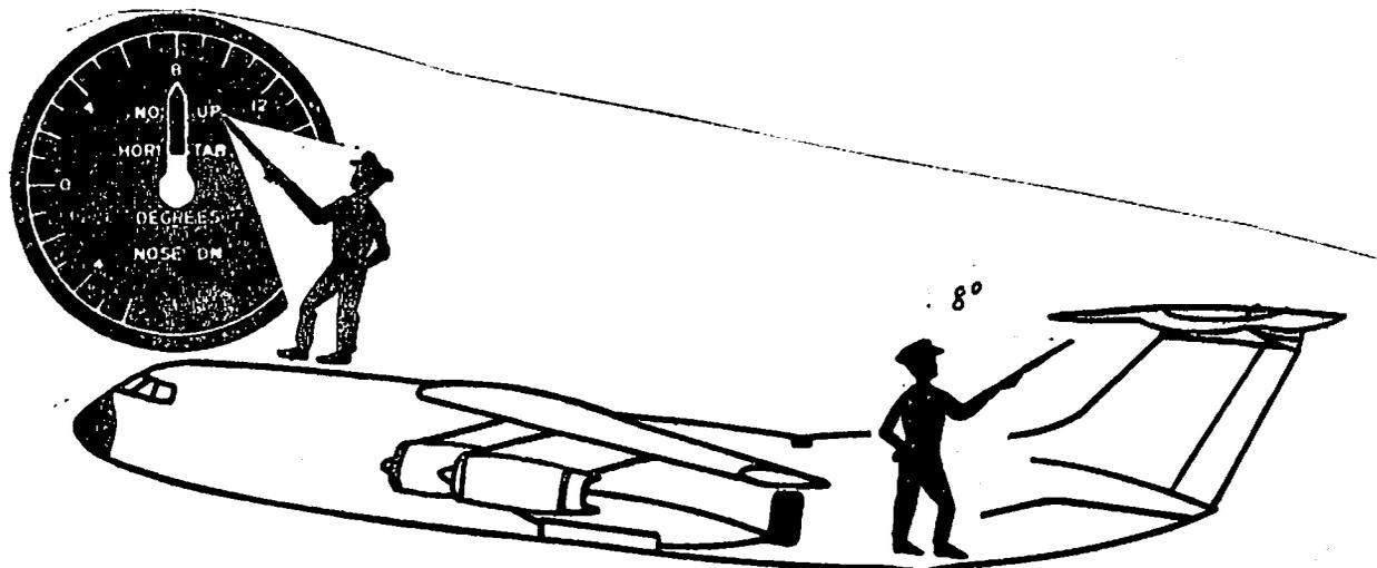
The indicator is indicating  $8^\circ$  nose up. This is the limit of travel for:
