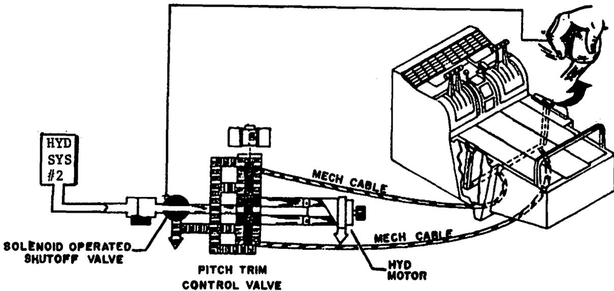
Depressing the button of either lever and pushing the lever forward will give
