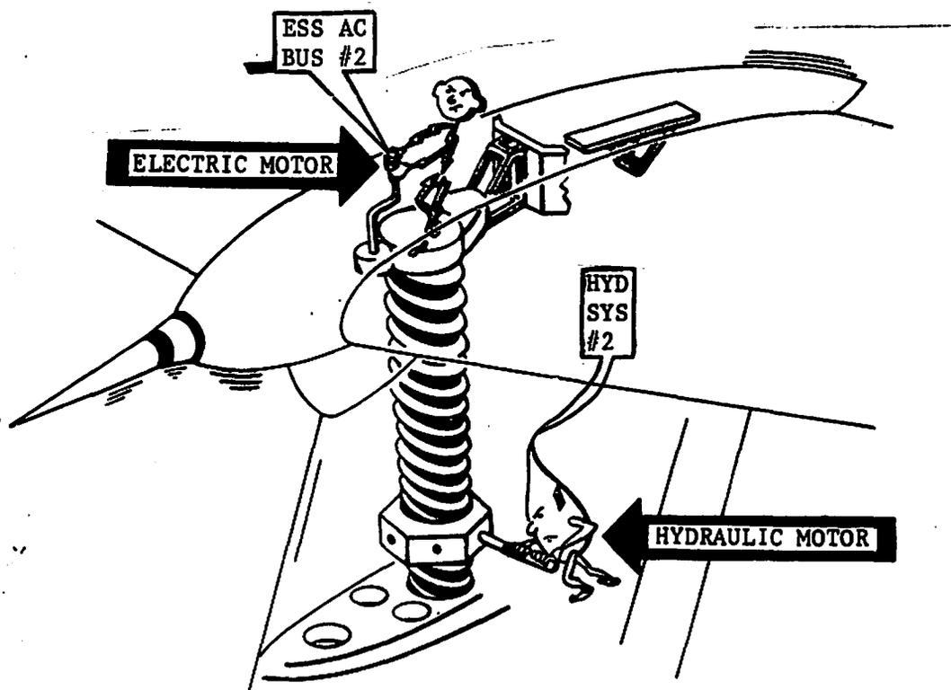
The Horizontal Stabilizer actuator is driven by a/an
