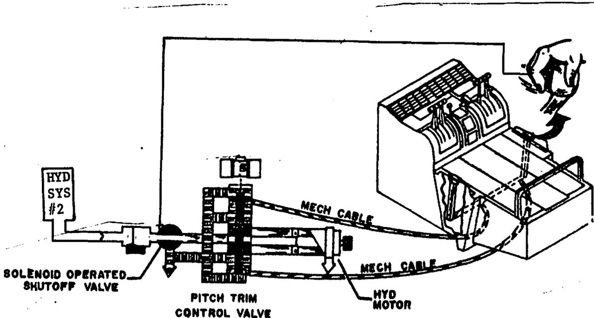
Notice there are two levers, one on each side of the center control pedestal. They are interconnected so both levers move together. The levers are also spring loaded to the center (OFF) position. Moving the lever forward will give nose down trim. Moving the lever aft will give nose up trim.
