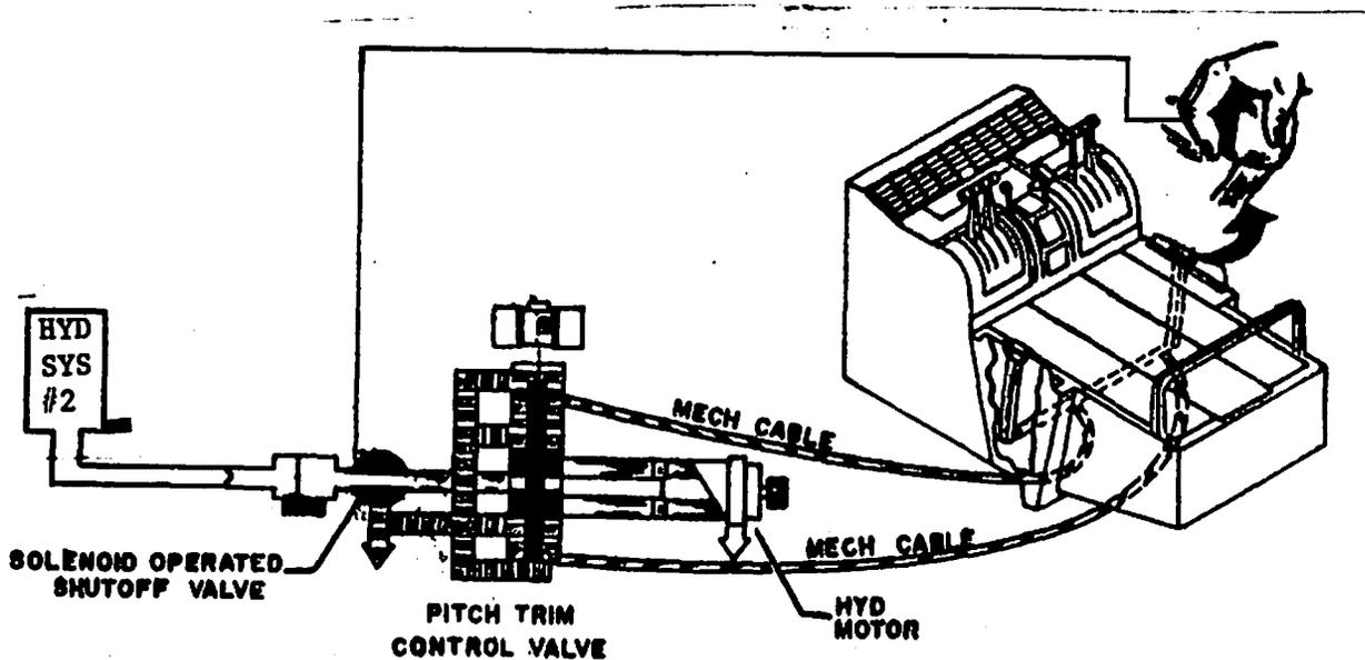
Will the Hydraulic Pitch Trim Levers be operational without electrical power?
