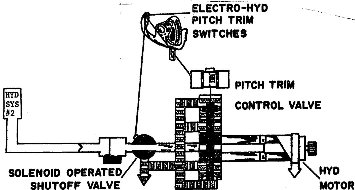
Does Electro-Hydraulic identify electrical control of hydraulic motor operation?
